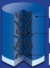
Copper oxide rods held together in wax matrix
